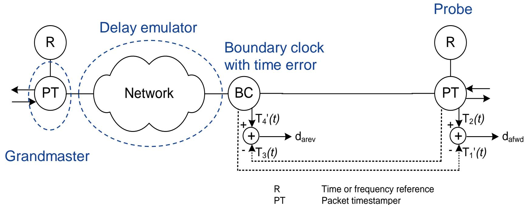
Measurement delay files,  $d_{afwd}(i)$  and  $d_{arev}(i)$ , are used to determine BC time error
